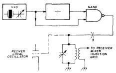
fig. 1. Rock-mixer block diagram. Circuit features surplus crystals and readily available ICs. The value is determined by formula to produce a synchronizing pulse train for the receiver LO. the crystal frequency, then the fre-Guency to which the crystal must be VXOed to receive 14062 kHz is 14997.818 kHz. By VXOing the 15000-kHz crystal to 14997.818 kHz and setting the divide-by-*n* circuit to 21, a pulse train of 15712 kHz will be
